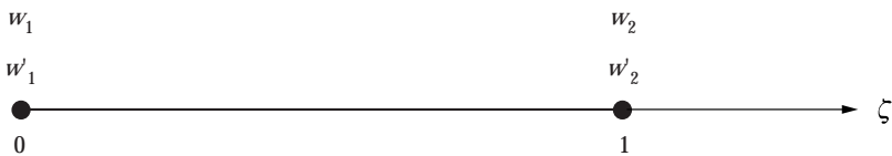
Figure 3. A 2-node reference beam element of four degrees of freedom.
